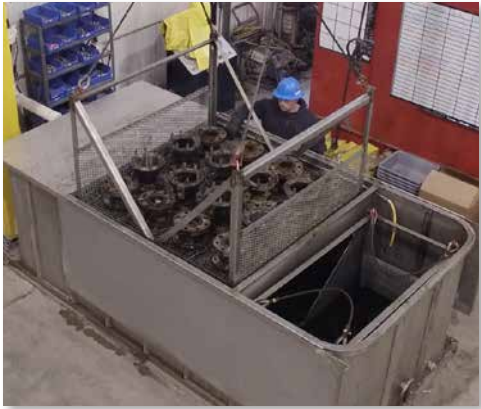
Removal of paint & petroleum residue
